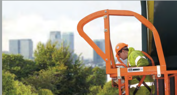
SanctuaryZone prevents the operator from being crushed
